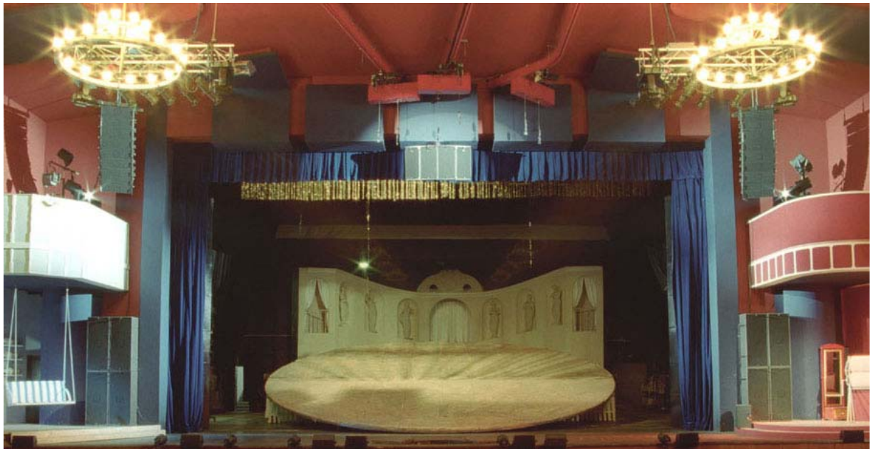
Figure 34: Flown ARCS center cluster (dV-DOSC L/R FOH)
