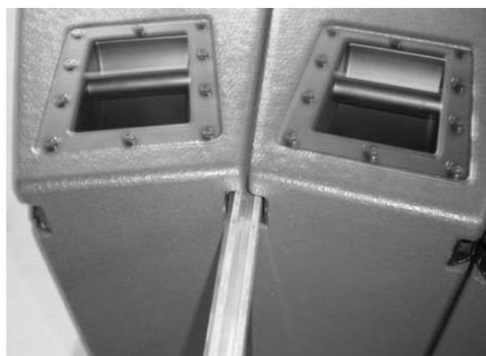
(6) ARCOUPL slides in from the rear of the array (two required, top and bottom)
