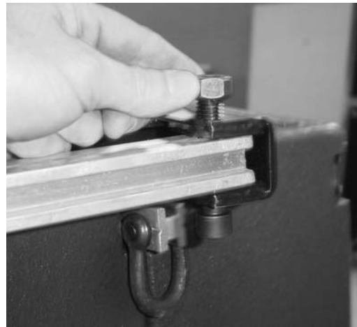
(10) ARCOUPL attached to the main body of the LIFTBAR at the rear
