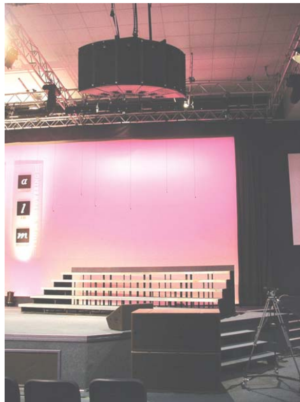
Figure 26: Single Row ARCS Array Examples
